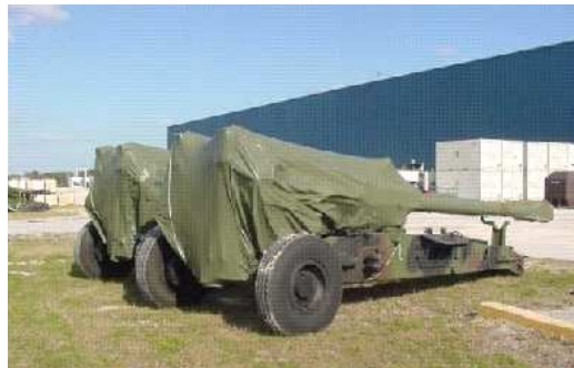
Figure 1: Image from Transhield commercial literature illustrating cover on the body of a howitzer. (Transhield, The Shrinkable Fabric (2006) www.transhield-usa.com/military.html )
