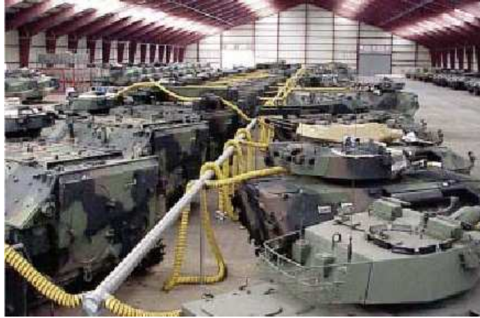
Figure 2: Example from J.H. Martin of equipment receiving dry air through manifold system and vehicle interface adapters at Marine Corps Logistics Base, Albany, Georgia. (Martin, J.H. (2005). Atmospheric Corrosion Suppression Through Controlled Humidity Protection — An Operational Readiness and Force Multiplier. Materials Performance , 61, 38.)
