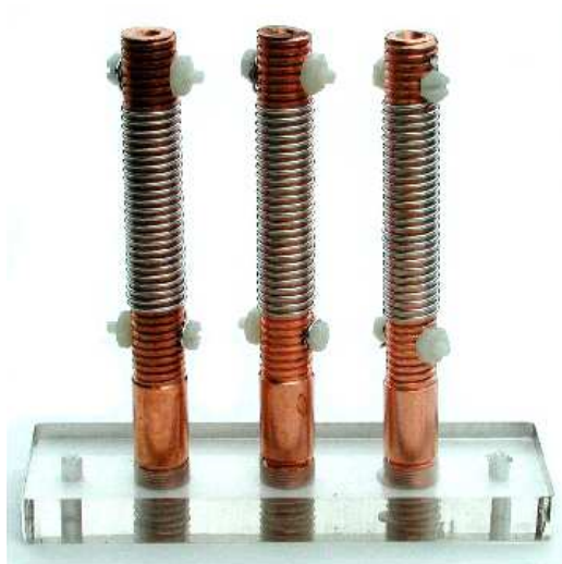
Figure 3: CLIMAT unit with three bolts of copper with aluminum wire.
